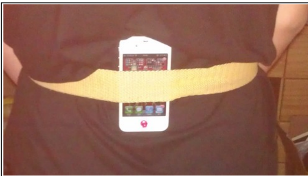
Fig. 2. Example of gait data collection by a smart phone
